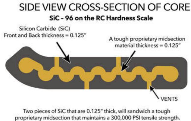
Body armor construction is composed of two pieces of SiC that are 0.125" thick, sandwiches a tough proprietary midsection that is 0.125" thick and maintains a 300,000 PSI tensile strength. This method allows for three-dimensional free-form shapes that can follow all body contours for maximum protection.
